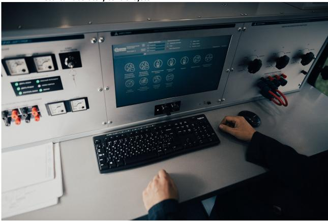
The Control System (CS) for ANGSTREM cable test van modules provides centralized control over the testing processes, localizing damages, various measurements, as well as the performance of service functions.
