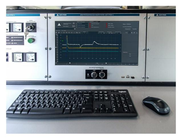
Designed to measure the cable line length, the distance to the place of damage to insulation and to determine the nature of a damage. It has a three-phase connection function. It supports all known non-burning methods. PC-based control.
